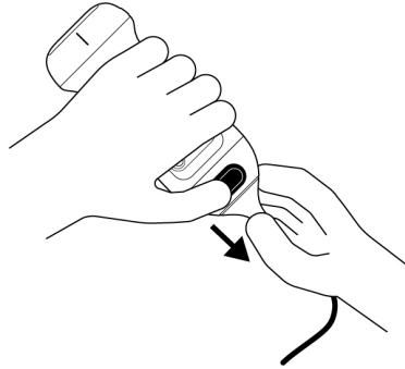
Figure 5. Removing the Butterfly iQ3 cable
