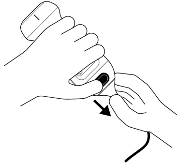
Figure 5. Removing the Butterfly iQ3 cable
